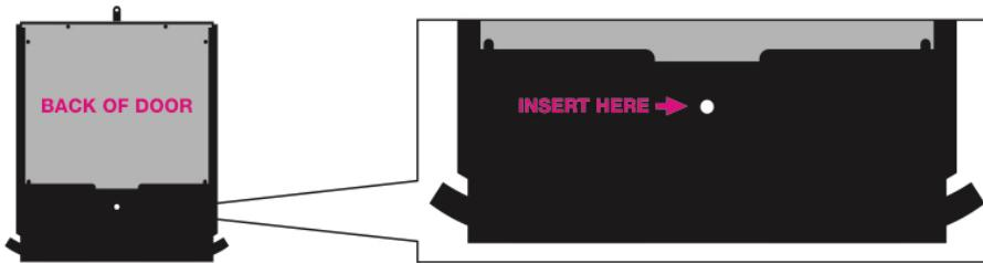
If worried about the locking mechanism freezing shut in extreme cold weather, this can be dis-engaged - simply ensure the door is in the fully up position, then insert a pin/screw/matchstick (not included) into back of unit to disengage locking mechanism. Door will now run freely without wings locking. Please remember to remove pin in order to re-activate when appropriate. Runners can also be lubricated in order to run freely in extreme weather.
